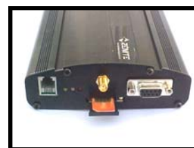
Picture 3.2: Inserting chip into connector
